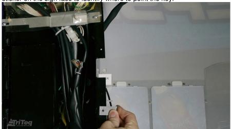
In a final example, the receiver is mounted inside the product delivery chute. The key will be pointed into the product delivery chute to operate the lock.
