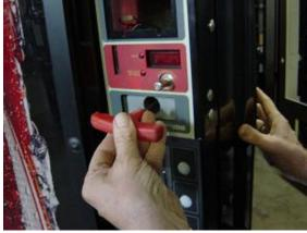
**Step Fifteen:** Install the T handle blocker
