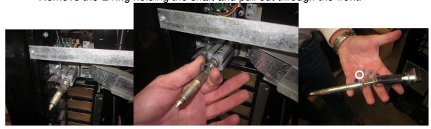
**Step Two:** Prepare the old T handle housing for the lock
